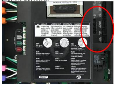
5) Disconnect the power wires from the electrical heater (Black, red, green and white cables) and secure the loose ends to a nearby ground stud.
