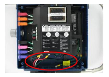
6) Connect one wire jumper to P63 and the other wire jumper to P66. Connect the wire jumpers to the two unmarked terminals of the relay
