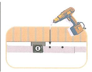
When both screws have been inserted and both sides still have a 1 1/2" clearance between the inside edge of the side arm and the spa side, you may want to lock the positioning by inserting an additional self-taping screw (if necessary to eliminate any horizontal sliding) to either side of the mounting blocks.
