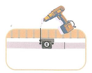
These "self-taping" screws will secure the bridge arm to the corner pieces.
