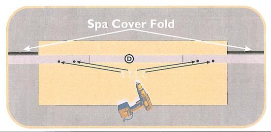
Before you fasten the screws, make sure the distance between the top comer pieces is the same as the distance between the bottom corner pieces. Also be sure you can see the Bridge Arm through each of the four screw holes. This will ensure that the screws will be
