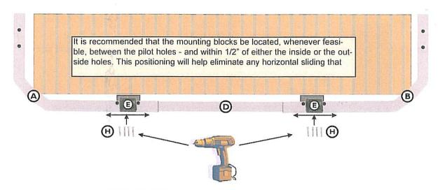
Any part of the spa frame that lines up correctly is OK. However, because it may not be possible to attach the mounting blocks to the spa frame, you might need to attach the mounting blocks to the deck or patio. If these options are not feasible, you can always use the Universal Mounting Kit. This kit provides flat aluminum plates that extend from under the spa and allow you to attach the mounting blocks to them. This kit is especially convenient if your spa is round or oval.
